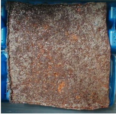
Figure 5 Marine Steel Pressured Washed, Then Abrasive Blasted Exposed to Humidity 6 years later
