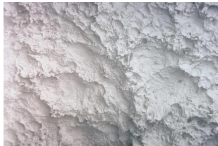
Figure 2 Water Jet Cleaned-Rounded Initial Profile
